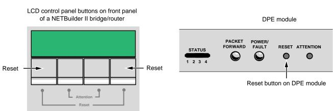
Push both reset buttons simultaneously
